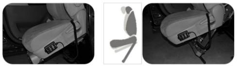
II. Then TRAVEL the seat back using the <sup>1</sup>/<sub>4</sub> inch hex tool (ratchet) in the outer hole and turn CLOCKWISE until the seat is level. Then simply follow the aforementioned steps.
