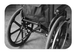
Remove either 'pin' from the end of the upper cylindrical tube and slide it out from within the bracket. For the lower cylindrical tube, you must remove both 'pins'. Once you have done that, slide the cylindrical tube to the left or right until the one side is free, then simply slide out the other side. Your wheelchair is now ready to be folded.
