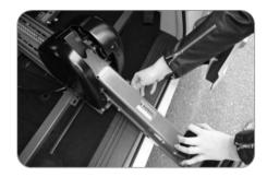
2. Press and hold down the release handle and push the SPEEDY-LIFT back into the vehicle.
